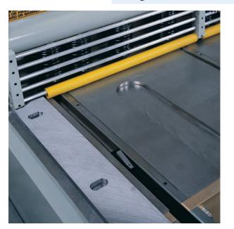
Gauge stops located on 24" centers travel 24" front to rear in unison. This yields a total gauging range of 72", 120" or 144" with the operator selecting the proper stop. Indicator on the display panel designates which stop to use depending on the dimension programmed. Air finger option elevates only the correct finger.
